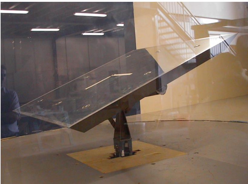
Image 13 - Wind Tunnel examination of a Reflector
